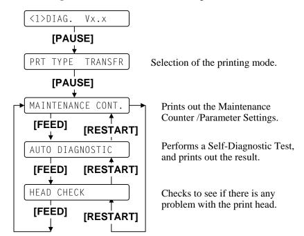
While pressing the **[FEED]** and **[PAUSE]** keys at the same time, turn on the printer. Hold both keys until the "<1>DIAG." Message appears in the display.
